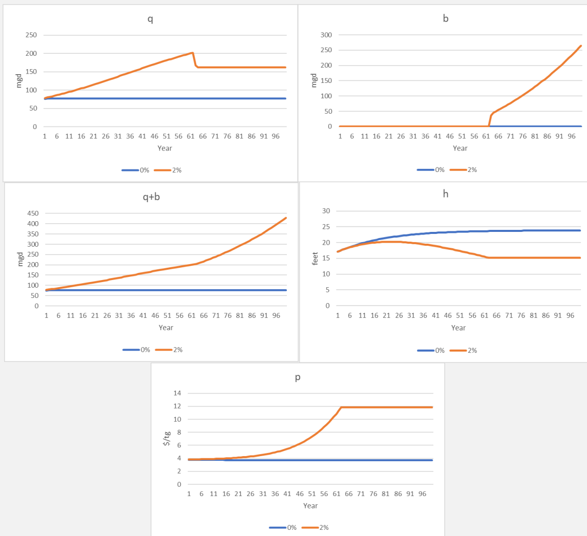
Figure 5: Optimal Trajectories for Groundwater Extraction, Desalination, Total Water Consumption, Efficiency Price, and Head Level for the Cases of 0 Percent and 2 Percent Annual Demand Growth
